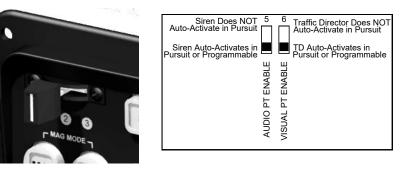
PROGRESSIVE ENABLE (Progressive Slide Switch Enable) Normally the slide switch is "progressive", meaning that each position will add another function while keeping the previous one(s) on. Position ① activates the first function. Position ② activates the functions connected to both ① and ②. Position ③ will activate all of the functions connected to ①, ②, and ③.
