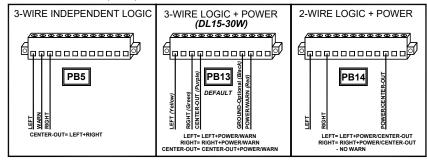
By default, when you set Control Head DIP switch #8 (DISCRETE TD) up (to use a LOGIC controlled TD), the output of the wires will control our DL15-30W (see center diagram above).
